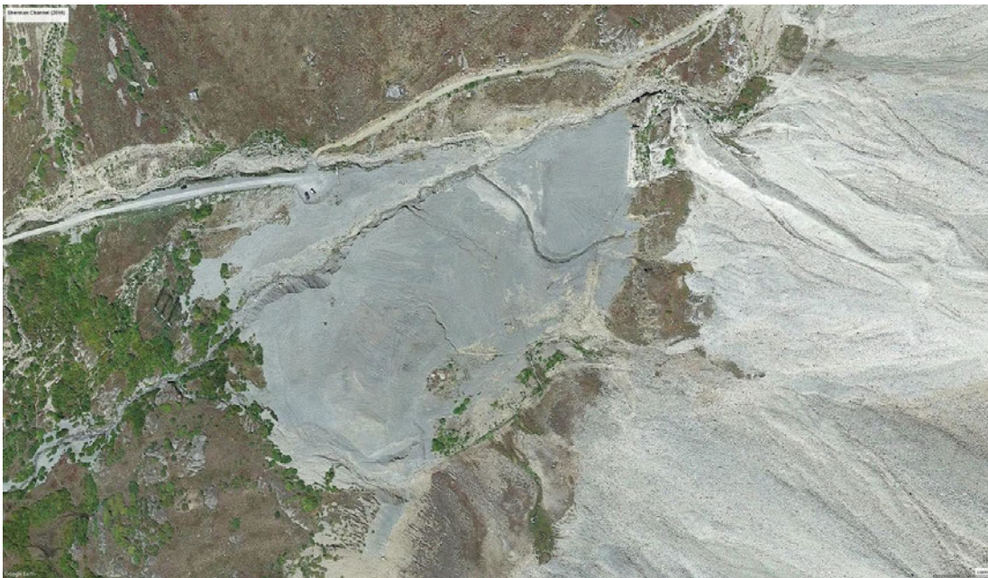
Figure 5. Aerial imagery showing extent of the site and available material that can be mobilized. This erosive environment needs to be stabilized to reduce sedimentation that can be seen in the receiving wetland. The event of 2008, where 10,000 CY of sediment was mobilized, could occur again, given recent climatic trends. Installation of this channel network will help stabilize the site long term.
