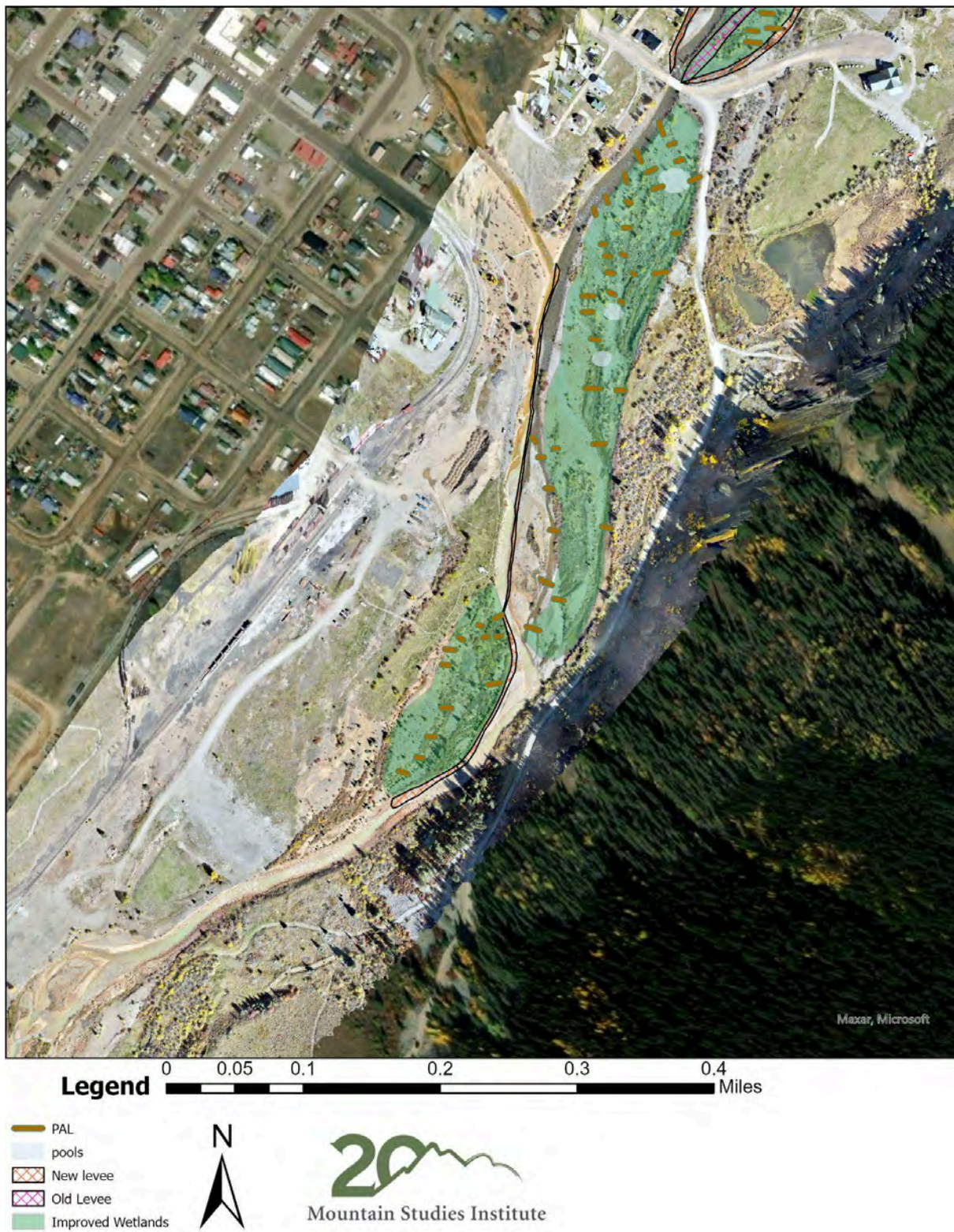
Figure 6: Design for instream and riparian wetland restoration of the lower half of the reach in Silverton.
